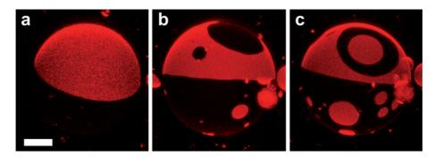
**Fig. 4** 3D confocal scans of the lower vesicle hemisphere illustrating lipid mixing induced by AC field (80 kHz, 500 V cm<sup>-1</sup>), at an external conductivity of 250  $\mu$ S cm<sup>-1</sup>. The vesicle (~95  $\mu$ m diameter) was prepared from a mixture of 2.66 : 5.33 : 2 DOPC : DPPC : Chol. Before applying the field (a), the vesicle has only two domains, which break apart after continuous field exposure of 2 min (b) and 3 min (c). The scale bar corresponds to 25  $\mu$ m.
