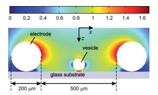
**Fig. 2** Electric field distribution at 100 kHz in a cross section of the chamber, passing through the centre of the vesicle. The vesicle is 40  $\mu$ m in radius and is located at 8  $\mu$ m above the glass. The media conductivity is 300  $\mu$ S cm<sup>-1</sup>. The field inside the vesicle is not calculated. The data are rescaled with the strength of a field, which would be induced between two parallel planar electrodes at a distance of 500  $\mu$ m.
